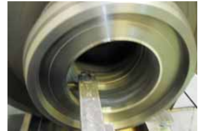
Bearing under rough machining
