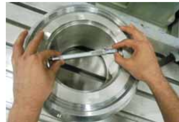
Dimensional check of bearing after machining
