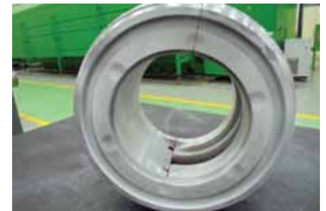
During NDT Test- No Pin Holes
