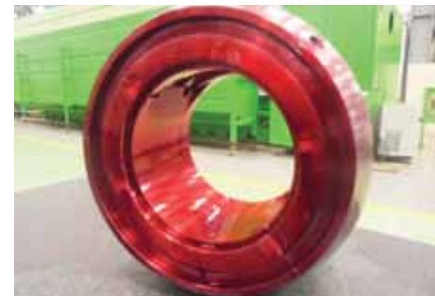
NDT test of Bearing
