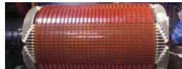
Rewinding of 11,000HP cylindrical synchronous rotor for Saudi Aramco
