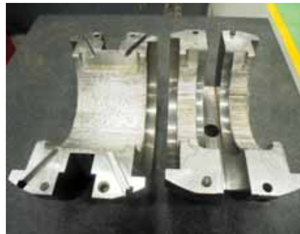
Bearings after welding process completed
