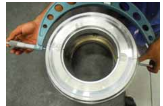
Dimensional check of bearing after machining
